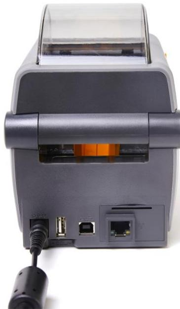
2. Connect the **power cord** to the power supply and an electrical outlet.
