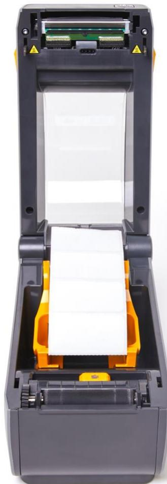
4. Pull the **labels** out past the cutter at the front of the printer.
