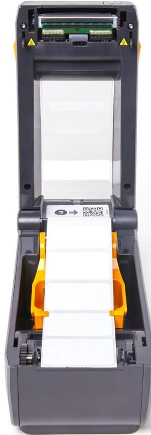
6. Flip the **labels** up and align the **movable sensor** to the centre position.
